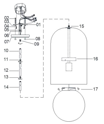
Components 01. Mounting Bar w/Green Screw 02. Mounting Screws 03. Hex Nut (8/32) 04. Outlet Box Mounting Screws 05. Hex Nut (1/8IP) 06. Lock Washer 07. Canopy 08. Cylinder Nuts 09. Nipple 10. Rod 11. Coupler (Dual-Head 1/8IP) 12. Rod 13. Coupler (Dual-Head 1/8IP) 14. Rod 15. Fixture 16. Glass holder 17. Glass Shade
